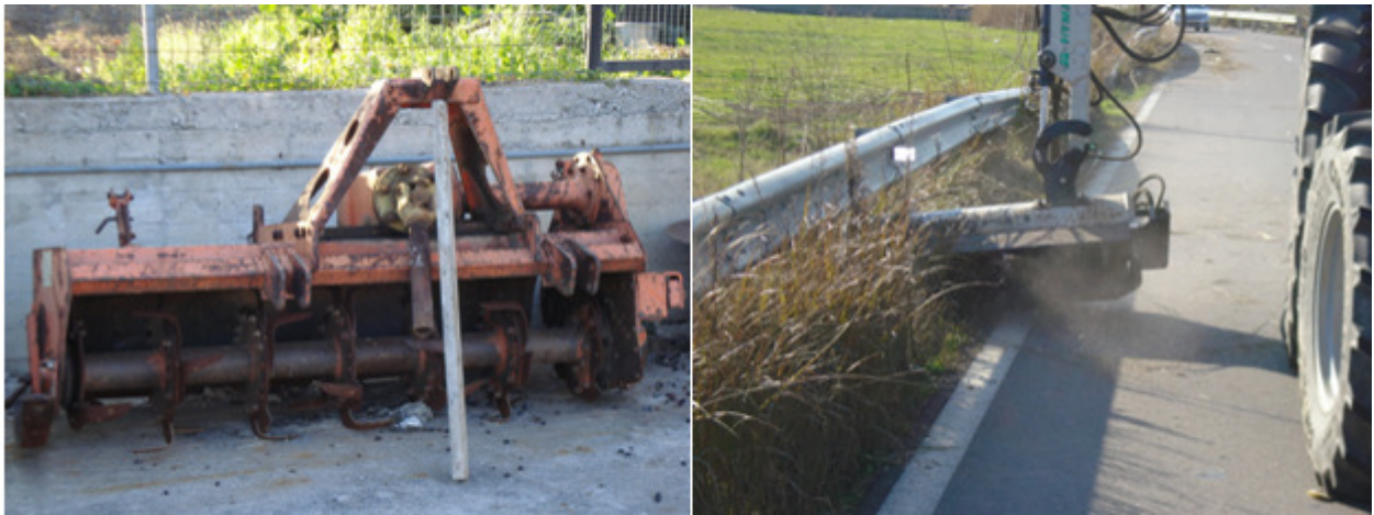
Figure 4.22: Machines used for clearing ground vegetation in Elia. The plowing machine is illustrated on the left frame, while the so-called “destructor” on the right.
