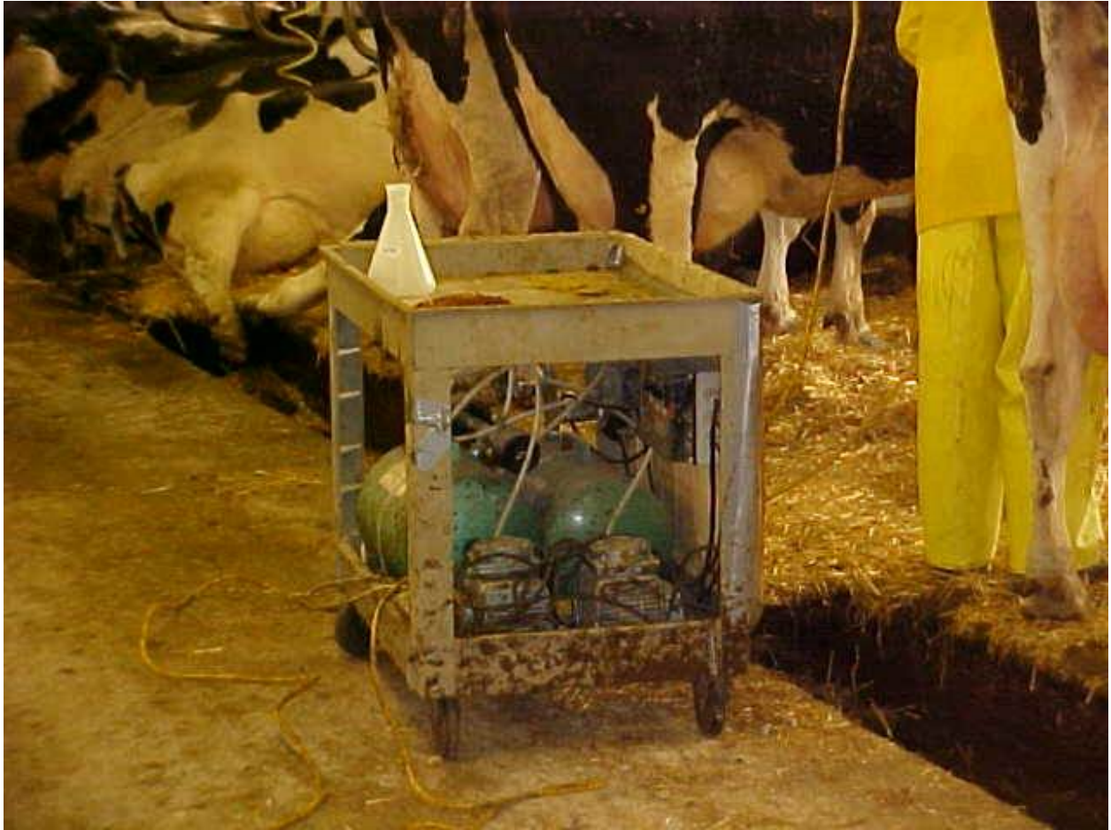
Figure 7: Dual vacuum pump (alternates pressure and vacuum) cart view.
