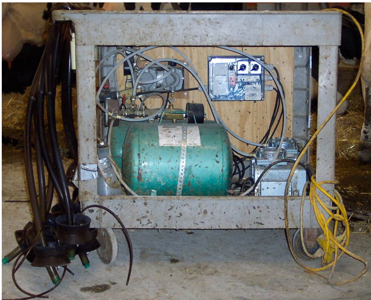
Figure 6: Dual vacuum pump (alternates pressure and vacuum).
