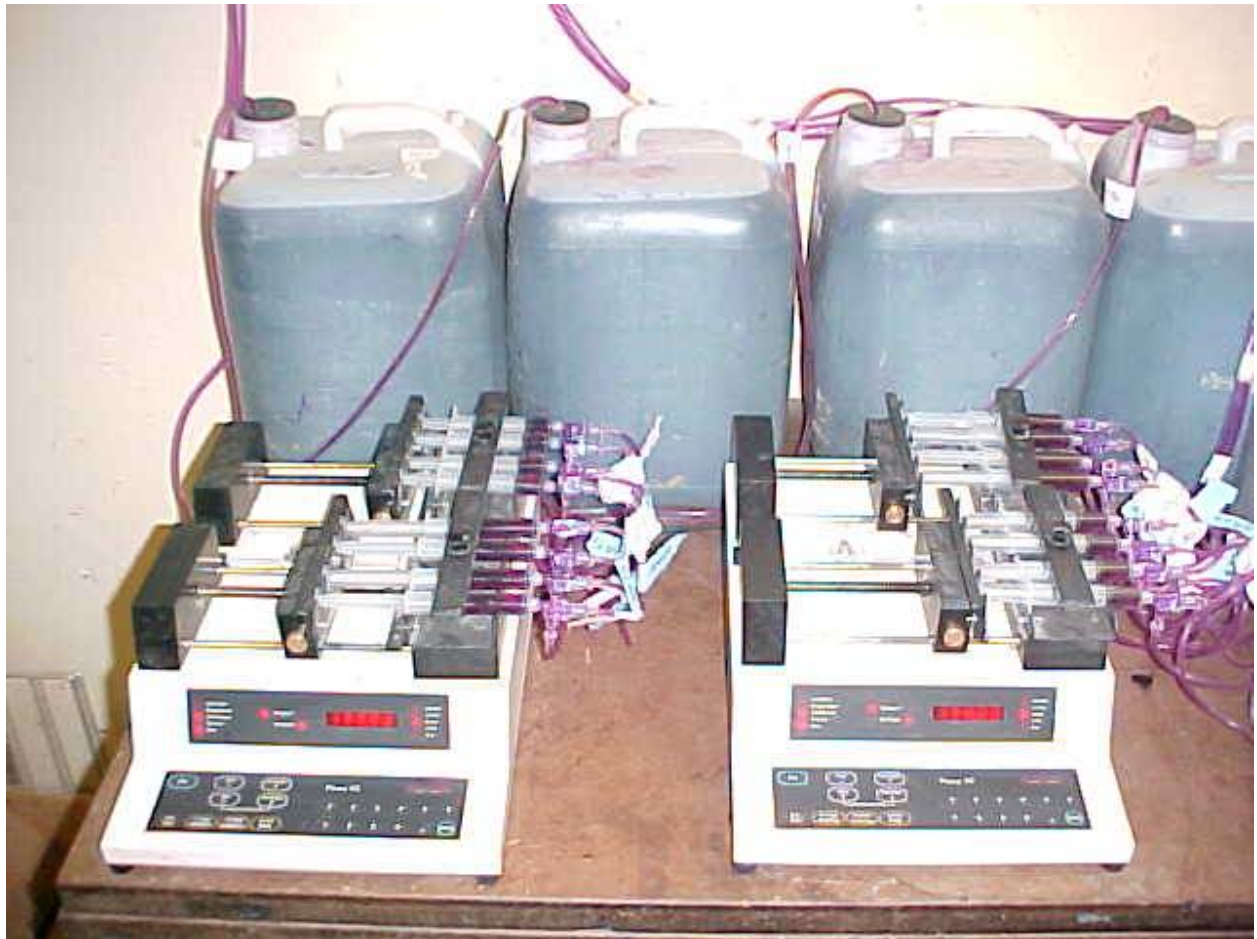
Figure 8: Triple-marker solution and syringe pump for infusion.
