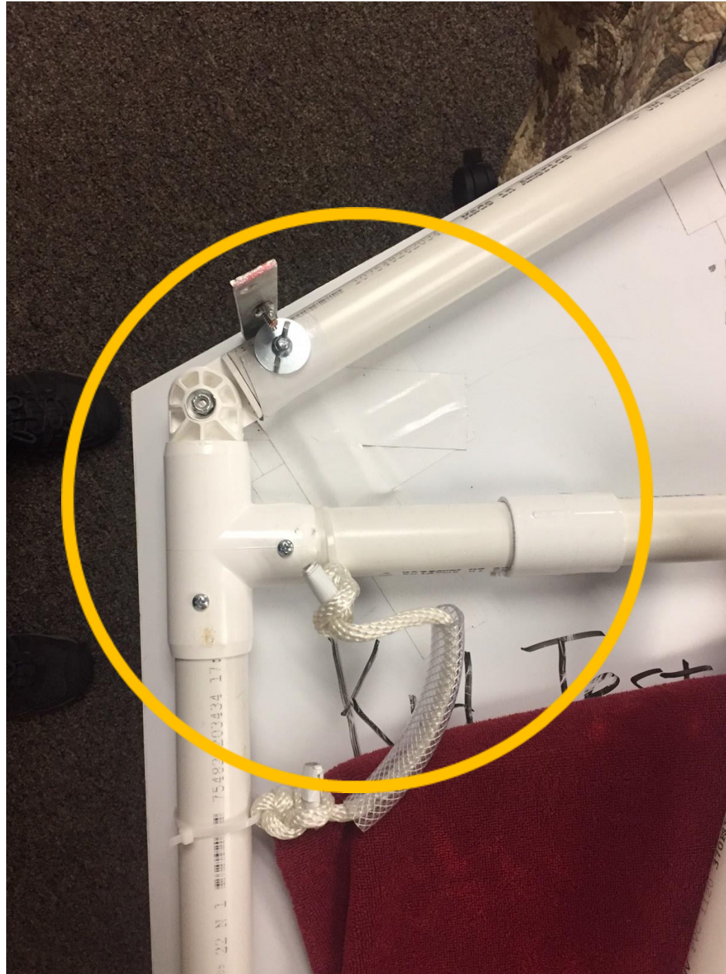
PVC frame upper corner showing the Tee and Adjustable Elbow joint, 5" Metal "L" Bracket (to attach roof section to) with bolt, fender washer and wingnut, spacer, and handle.
