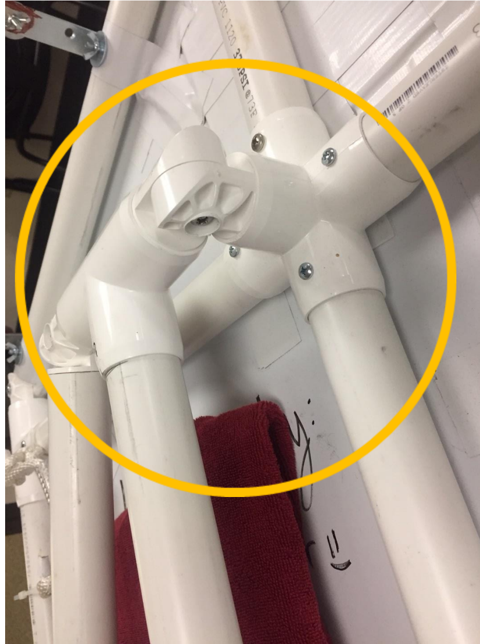
Upper Brace connection to the Main Frame in closed position showing the Five-way Cross, Adjustable Elbows, and Tee.
