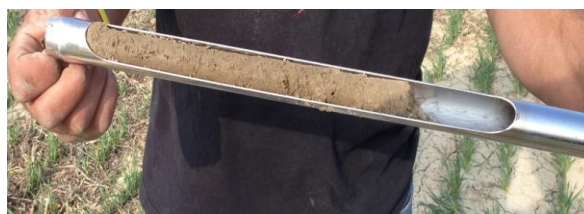
Figure 5: Soil sample collected by using soil probe. Photo by Maninder K. Walia.
