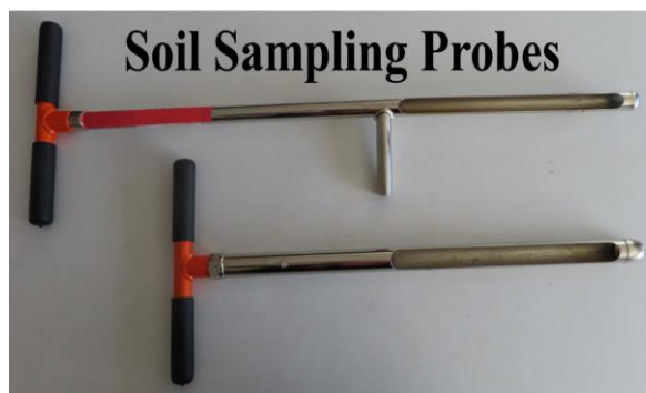
Figure 2: Soil samples can be collected by using probes. Photo by Maninder K. Walia.
