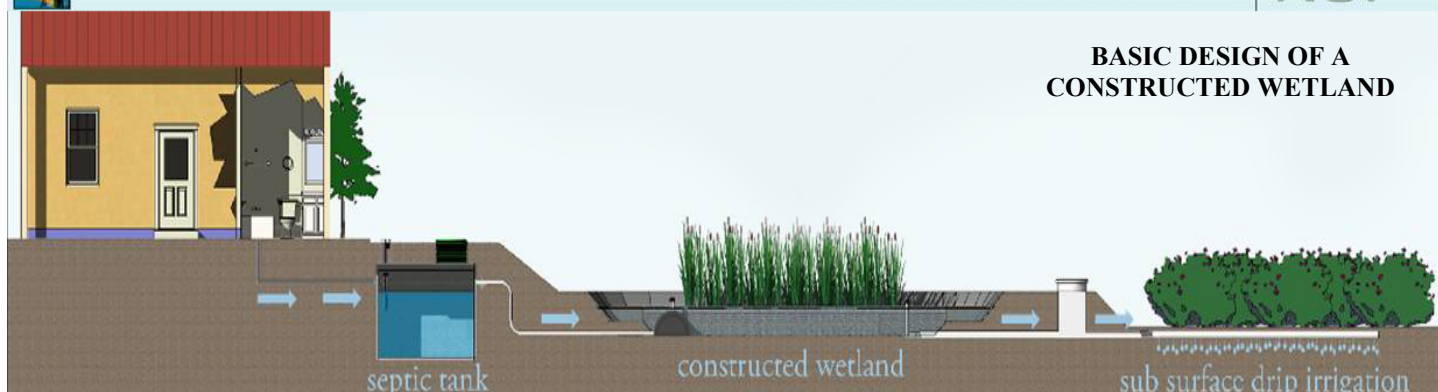
Fig. 5 A basic wetland design for home or business including black water (M. Ogden NSI)
