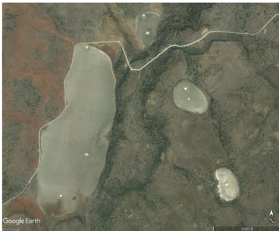
View of four Wet Clay Basin sites, all with small dugout ponds or “dirt troughs”. Located off Buckhorn Road in northwest Nevada, near 40.906 N, -119.884 S. The light colored spots are the ponds, which hold water into the growing season while letting surrounding land dry out by lowering the water table. Map data: Google 2018.
