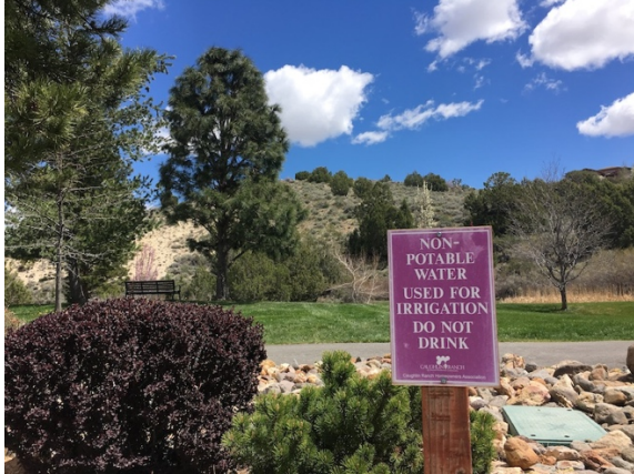
Figure 1. Typical purple compliance sign for reclaimed water used for landscape irrigation. The language and color signals nonpotable water quality.
