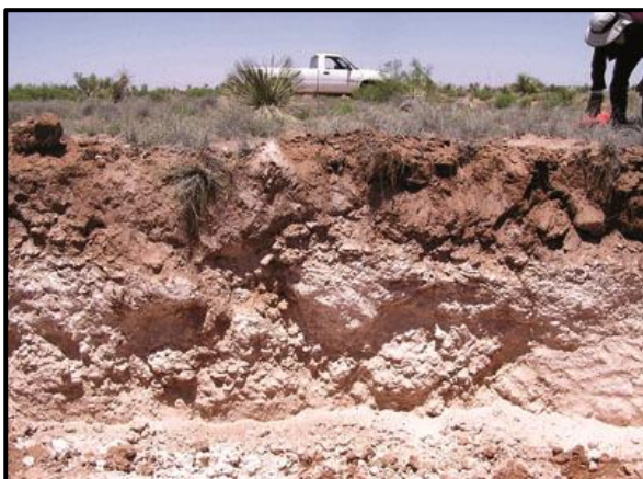
Figure 1. Common soil layers in arid regions, with poor water retention and high alkalinity. The topsoil contains fine sandy loam with light brown hues; transitions to deeper layers rich in calcium carbonate, known as caliche; with a hardpan forming at the lowest horizon. (Idowu and Flynn, 2015). Photo credit: Cheryl Kent.
