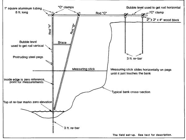
Fig. 2. The moveable frame set up.
